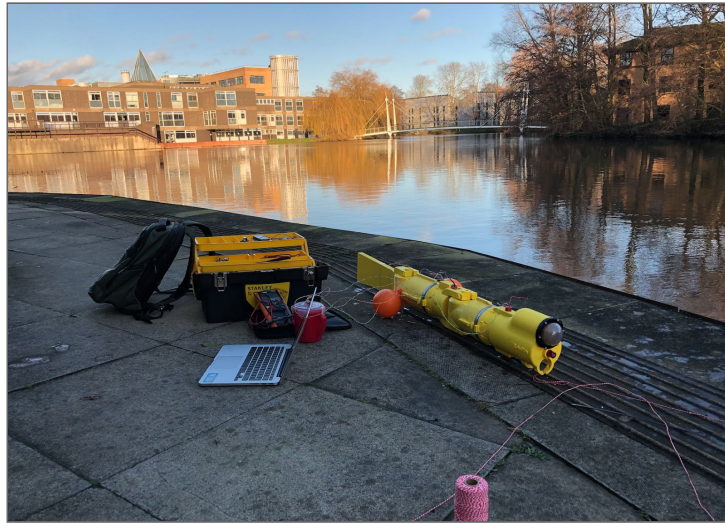
Fig. 6 the tested Robofish prototype with a head, tail and one segment
