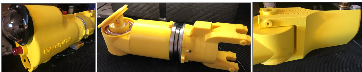
Fig. 3: Body Segments with Magnetic Joints, head and caudal tail fin
